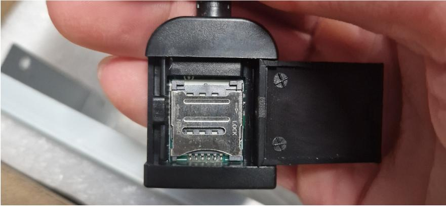
As you can see there is a small gap on the metal plate, you will need fingernails to lift it up, under this will be some metal pins, that the SIM card is placed into.
