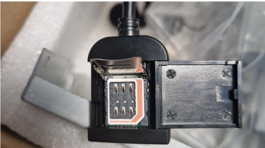
Once that is placed in, ensure that the metal side is face down, otherwise, no connection to the PINS will be established, and it won't work.
