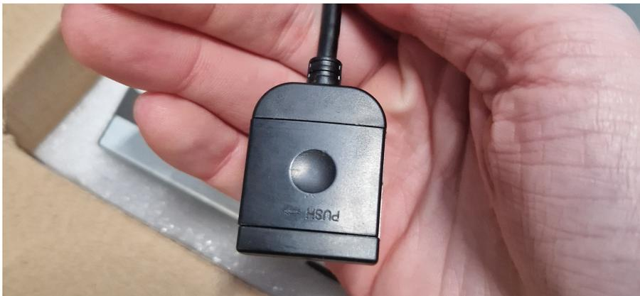
**Step 3:** Similar to a television remote, you will be able to push the side of the SIM card holder open as if you were removing the batteries from a television remote.
